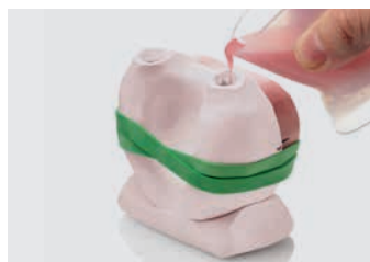
12. Pour the resin into one of the two pouring channels
