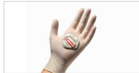
3. For each measure, spread two strips of Zhermack Indurent LAB catalyst the same length as the measure, i.e. about 4 cm
