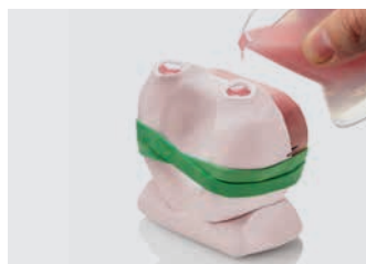
13. The pouring is complete when the resin oozes out of the opposite channel
