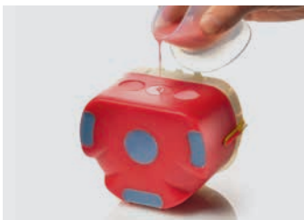
13. The pouring is complete when the resin oozes out of the side channels
