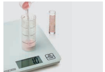
11. Weigh the resin, measure the monomer and mix, pouring the monomer in first and then the resin
