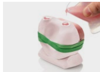
13. The pouring is complete when the resin oozes out of the opposite channel
