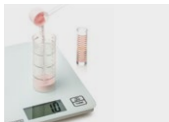
7. Weigh the resin, measure the monomer and mix, pouring the monomer in first and then the resin
