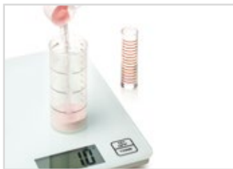
1. Weigh the resin and measure the monomer. Mixing ratio: 10 g of resin and 6.7 g (7 ml) of monomer
