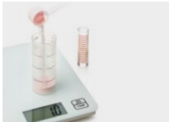
9. Weigh the resin, measure the monomer and mix, pouring the monomer in first and then the resin
