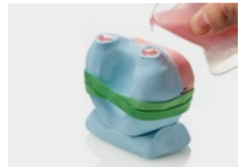
15. The pouring is complete when the resin oozes out of the opposite channel
