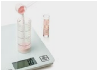
9. Weigh the resin, measure the monomer and mix, pouring the monomer in first and then the resin
