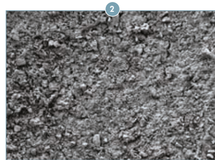
SEM* shows glazed porcelain surface AFTER 1-minute treatment with Pulpdent Porcelain Etch Gel. Note the microscopic tags in the porcelain surface.
